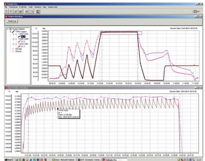
Typical test of hospital autoclave with 4 pre vacs.
